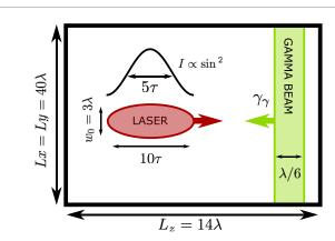
Figure 6. Typical set-up of the 3D PIC simulations, with  $\lambda$  and  $\tau$  the laser wavelength and the optical cycle, respectively.
