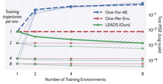
Figure 4: Test error for LV w.r.t. the number of envs. We apply the models in 1 to 8 envs. 4 groups of curves correspond to models trained with 1 to 8 trajectories per env. All groups highlight the same tendencies: increasing One-For-All , stable One-Per-Env. , and decreasing LEADS .
