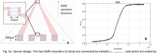
large pads to facilitate the connection. 2b – Typical, R(H) resistance response to an applied along the reference magnetization
