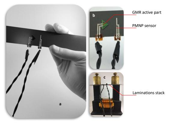
Fig. 3a – The instrumented ferromagnetic lamination, 3b – The non-invasive sensor, 3c – The sensor embedded in a lamination stack.
