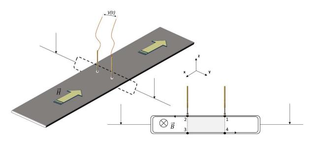
Fig. 1 – Magnetic needle probe method, explanation scheme.
