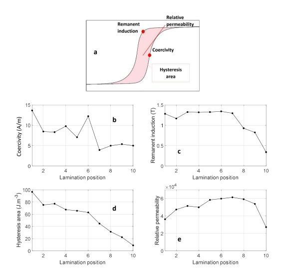
Fig. 7a – The hysteresis cycle parameters, 3b - Evolution of the coercivity as a function of the lamination position, <math>3c - Evolution of the remanent induction as a function of the lamination position, <math>3d - Evolution of the hysteresis area as a function of the lamination position, <math>3e - Evolution of the remanent induction as a function of the relative permeability as a function of the lamination position.
