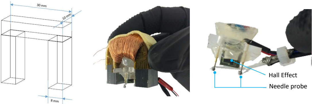
Fig. 6 – Magnetic Inductor; core dimensions (left), magnetic Inductor unit (middle) and magnetic sensors (right)
