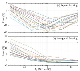
Fig. 7. Percentage error of the proposed model compared to FEA for (a) square-packed and (b) hexagonal-packed wires. Each curve corresponds to a particular combination of  $t_{\rm ins}$  and  $t_g$ .
