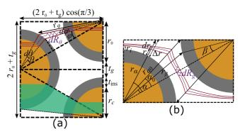
Fig. 5. Hexagonal-packed wires showing various thermal resistances. Thermal resistance is calculated for unidirectional heat flow from left to right. (a) A unit cell showing the infinitesimal thermal resistance  $dR_{\theta}$  given by (15) and (b) a half-unit cell showing the infinitesimal thermal resistance  $dR_g$  given by (25). The red enclosed areas show paths of integration.
