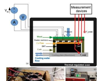
Fig. 9. Experimental test setup. (a) Test bench schematic, (b) test bench picture, and (c) instrumentations.
