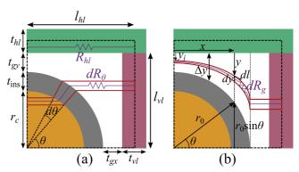
Fig. 4. A quarter-unit cell (black dashed box) of square-packed wires showing various thermal resistances. Thermal resistance is calculated for unidirectional heat flow from left to right. The red enclosed areas show path of integration for the infinitesimal thermal resistances (a)  $dR_{\theta}$  given by (5) and (b)  $dR_{q}$
