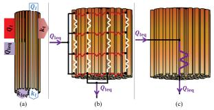
Fig. 12. Definition of litz-wire thermal conductivities. (a) Path of different heat sources, (b) transverse and longitudinal resistances, as a thermal network inside the litz wire, (c) definition of the longitudinal equivalent thermal resistance with conductivity  $k_{\rm leq}$  substituting the thermal network in (b).
