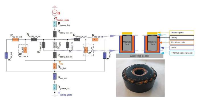
Fig. 14. Thermal network model for samples 3 and 5, showing thermal resistances corresponding to the core material (light grey), epoxy (dark grey), grease (light blue), resin (dark blue) and litz wire (orange). Litz-wire thermal resistances calculated using the equivalent longitudinal conductivity are surrounded by dashed rectangle; the other litz-wire thermal resistances are calculated using the transverse conductivity.
