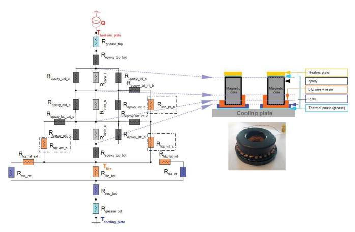
Fig. 13. Thermal network model for samples 1, 2 and 4, showing thermal resistances corresponding to the core material (light grey), epoxy (dark grey), grease (light blue), resin (dark blue) and litz wire (orange). Litz-wire thermal resistances calculated using the equivalent longitudinal conductivity are surrounded by dashed rectangle; the other litz-wire thermal resistances are calculated using the transverse conductivity.
