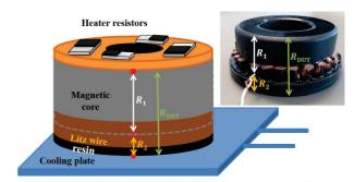
Fig. 10. Schematic of the samples showing measurements for thermal resistances  $R_1$ ,  $R_2$  and  $R_{\rm DUT}$ .
