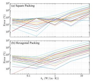
Fig. 8. Absolute value of the percentage error of the TEFA model compared to FEMM simulation for (a) square-packed and (b) hexagonal-packed wires. Each curve corresponds to a particular combination of  $t_{\rm ins}$  and  $t_g$ . The errors are plotted on the logarithmic scale. Points with very large errors correspond to cases with high gap thermal conductivity  $k_g$  and or large gaps (large values of  $t_g$ ,  $t_{gx}$ ,  $t_{gy}$ ).
