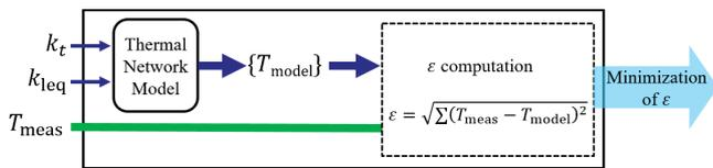
Fig. 15. Inverse problem for calculating the thermal properties of litz wire.
