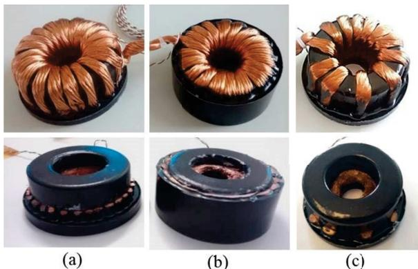
Fig. 11. Sample pictures. Top: before the litz wire cutting, bottom: after the litz wire cutting (used for measurements). (a) molded only at the bottom and 100% layer fill rate, (b) molded to the top and 100% layer fill rate, (c) molded only at the bottom and 66% layer fill rate.
