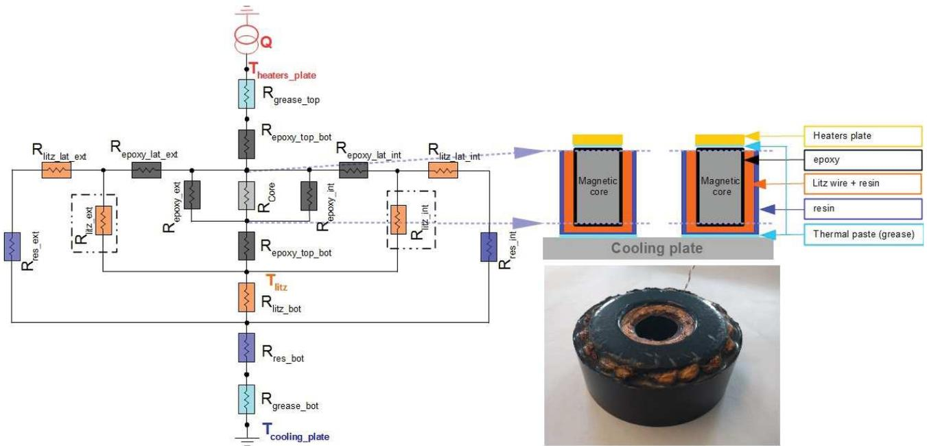
Fig. 14. Thermal network model for samples 3 and 5, showing thermal resistances corresponding to the core material (light grey), epoxy (dark grey), grease (light blue), resin (dark blue) and litz wire (orange). Litz-wire thermal resistances calculated using the equivalent longitudinal conductivity are surrounded by dashed rectangle; the other litz-wire thermal resistances are calculated using the transverse conductivity.
