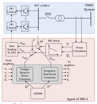
Fig. 2: Multi-layer control algorithms in an agent.
