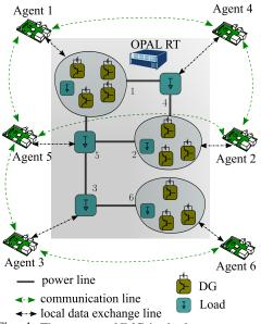
Fig. 4: The test case NMG in the layer structure.
