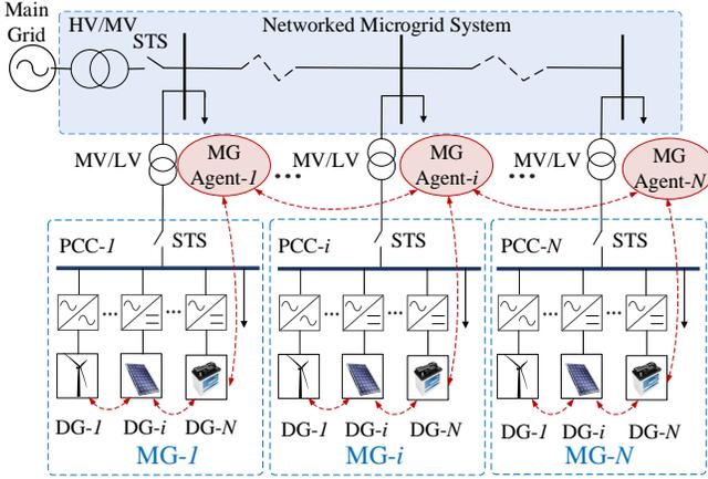
Fig. 1: Typical schematic of the networked microgrid systems
