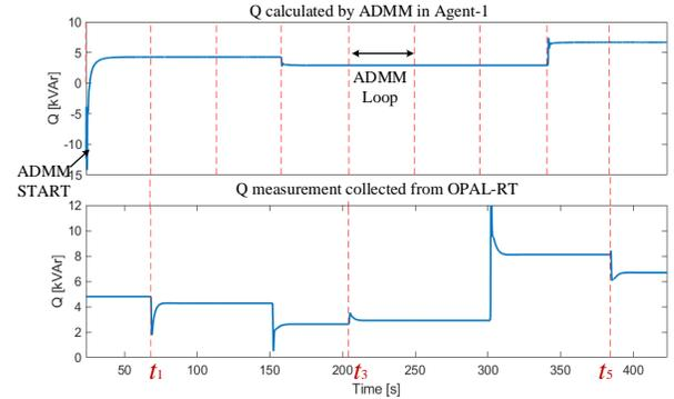
Fig. 11: Reactive power of MG-1 output calculated in Agent 1
