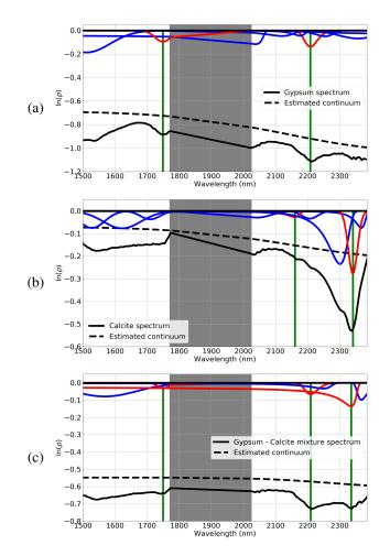
Fig. 12: Deconvolution of gypsum (a) and calcite (b) spectra, and a mixture of both (c). The true positions of the diagnostic and secondary absorptions are shown as vertical lines.
