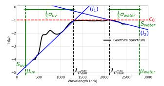
Fig. 2: Computation of the initial continuum parameters  $\theta_c^{start}$  for a goethite reflectance spectrum from the USGS spectral library [18]: sample splib07b\_Goethite\_GDS134\_ASDFRb\_AREF. The lines  $l_1$  and  $l_2$  are drawn in blue, and the maximum of the spectrum  $c_0$  is in dashed red. The parameters of  $G_{uv}$  and  $G_{water}$  are in green.
