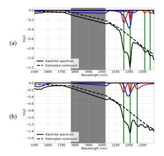
Fig. 13: Deconvolution of kaolinite spectra from two piles. The true positions of the diagnostic and secondary estimated absorptions are shown as vertical lines.
