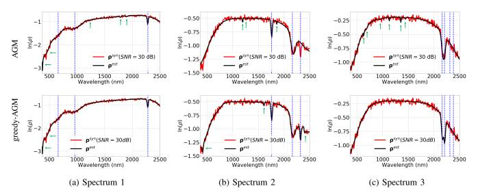
Fig. 4: Assessment of the AGM (top) and greedy-AGM (bottom) procedures for the three noisy synthetic spectra. Noisy and estimated spectra are shown in red and black, respectively. Synthetic absorption positions are represented as vertical dashed blue lines. Green arrows indicate the location of false EGO Gaussians.
