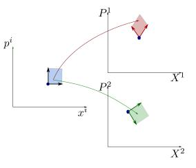
Figure 3. For a canonical transformation, the sum of a projected area in a given plane  $(x^i, p_i)$  into all planes  $(X^j, P_j)$ (j = 1...n) is conserved.
