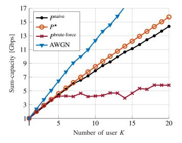
Fig. 4. Sum-capacity vs. number of users K with  $G_{amp} = 10 \text{dB}$ .
