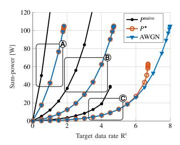
Fig. 1. Sum-power vs. target data rate  $R_k^t = R^t$  with  $G_{amp} \in \{-10, 0, +10\}$ dB (A, B and C respectively).
