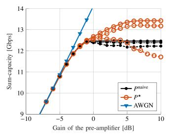
Fig. 3. Sum-capacity vs. pre-amplifier gain  $G_{\rm amp}$  with  $\epsilon \in \{30,50\}\%$  (in dotted and dashed line respectively). The solid line is the case of perfect channel gain estimation.
