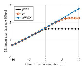
Fig. 2. Minimum of user data rate vs. pre-amplifier gain  $G_{amp}$ .
