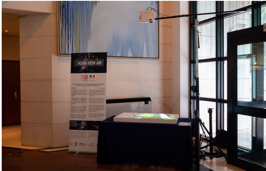
Fig. 5: The full setup for tangible and interactive simulations (including the 3D map, the tablet with the Android application, the projector).
