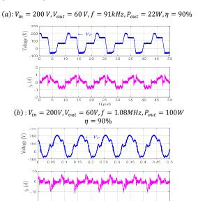
FIGURE 4. WAVEFORM OF VOLTAGE AND CURRENT OF PR NEAR RESONANT FREQUENCY FOR: (A) RADIAL MODE, (B) THICKNESS MODE.
