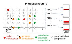
(b) Hybrid (discrete-time and discrete-event) approach for parallel simulation (at processor level)
