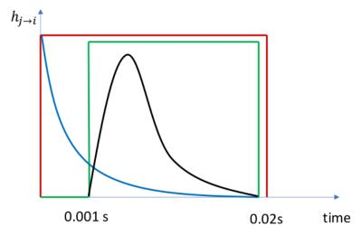
Figure 1: Examples of interaction functions  $h_{j\to i}$  from a neuron j to a neuron i: in red a piecewise constant function with no delay; in green a piecewise constant function modeling a synaptic transmission delay; in black a continuous interaction function with the same synaptic delay; in blue the exponential interaction function, obtained in the most classic Integrate-and-Fire models.
