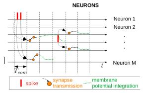
(a) Hybrid (discrete-time and discrete-event) approach for parallel simulation (at neuronal level)
