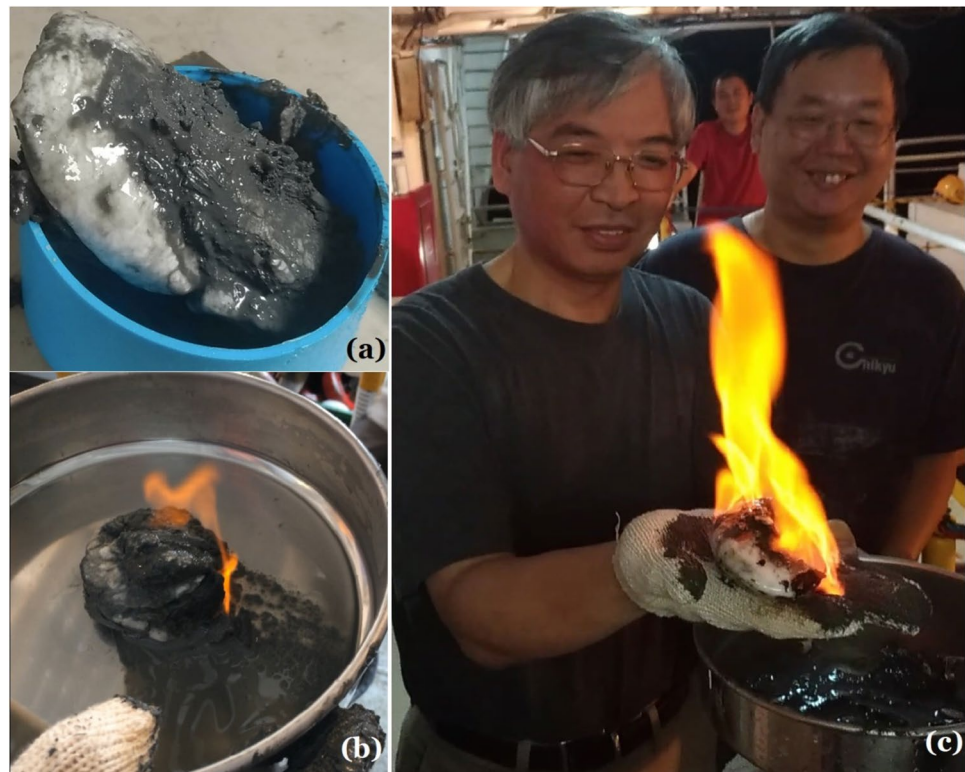
Fig. 3 a The gas hydrate sample collected at core site MD18-3542, and b the sample collected at core site MD18-3543. c The burning gas hydrate obtained at core site MD18-3542. The person who holds the burning gas hydrate is Prof. Shu-Kun Hsu, and next to him is Prof. Chih-Chieh Su
