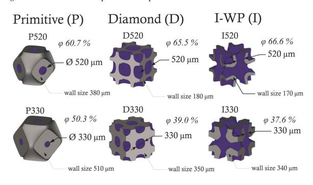
Figure 1. The basic cells parameters of different samples with TPMS architectures
