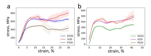
**Figure 4**. The stress-strain curves for Primitive, I-WP, Diamond structures with different minimal diameters of pores ( $a - 330 \ \mu m$ ;  $b - 520 \ \mu m$ )
