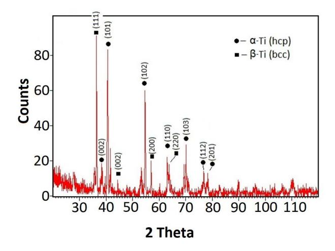
Figure 3. The XRD pattern of the Rematitan®CL titanium alloy after the SLM process and heat treatment
