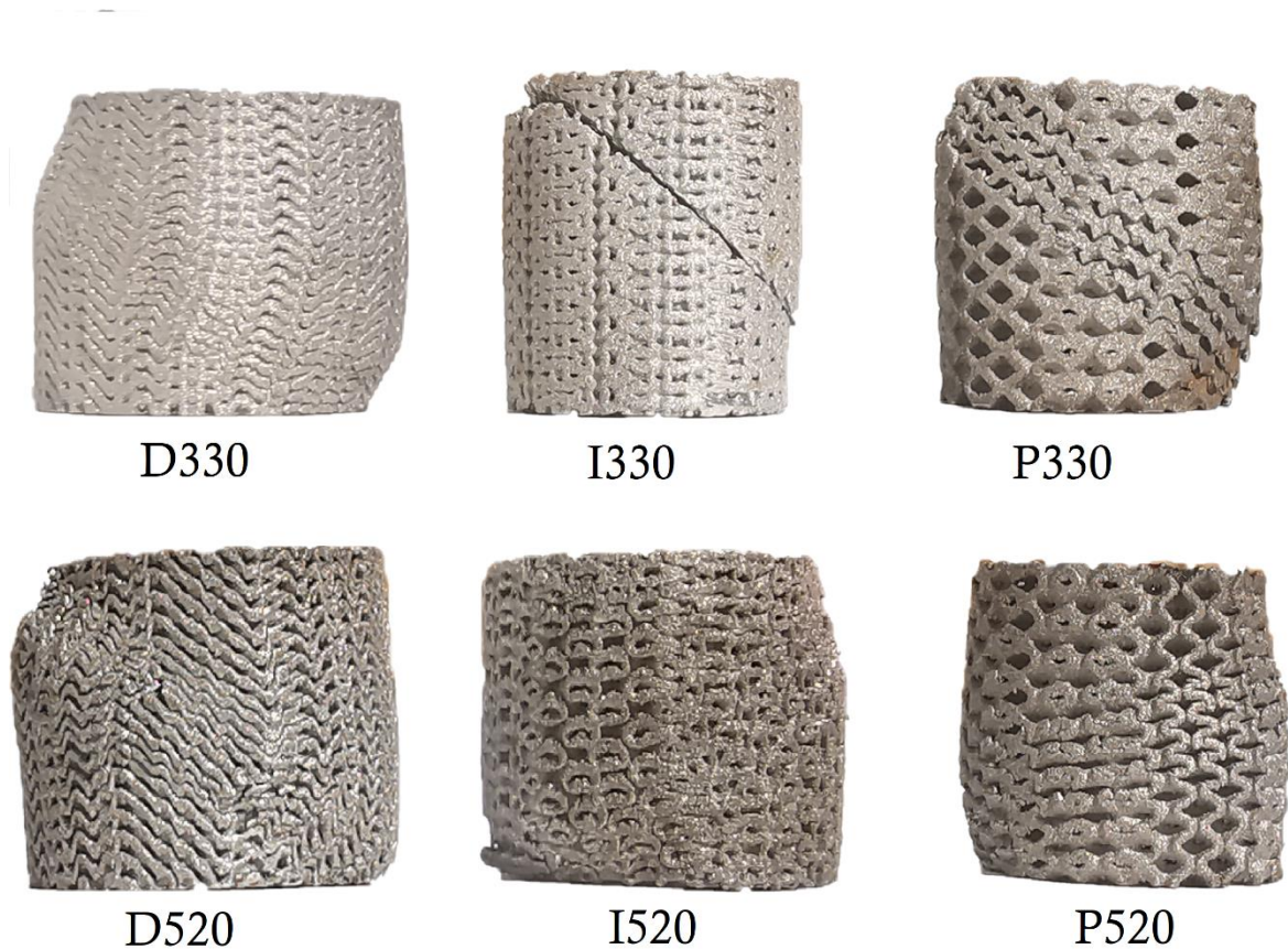
Figure 6. The destruction behavior of porous scaffolds with different architecture
