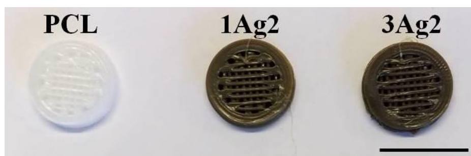
22 Figure 1. Photograph of the 3D printed scaffolds (scale bar denotes 1cm)
