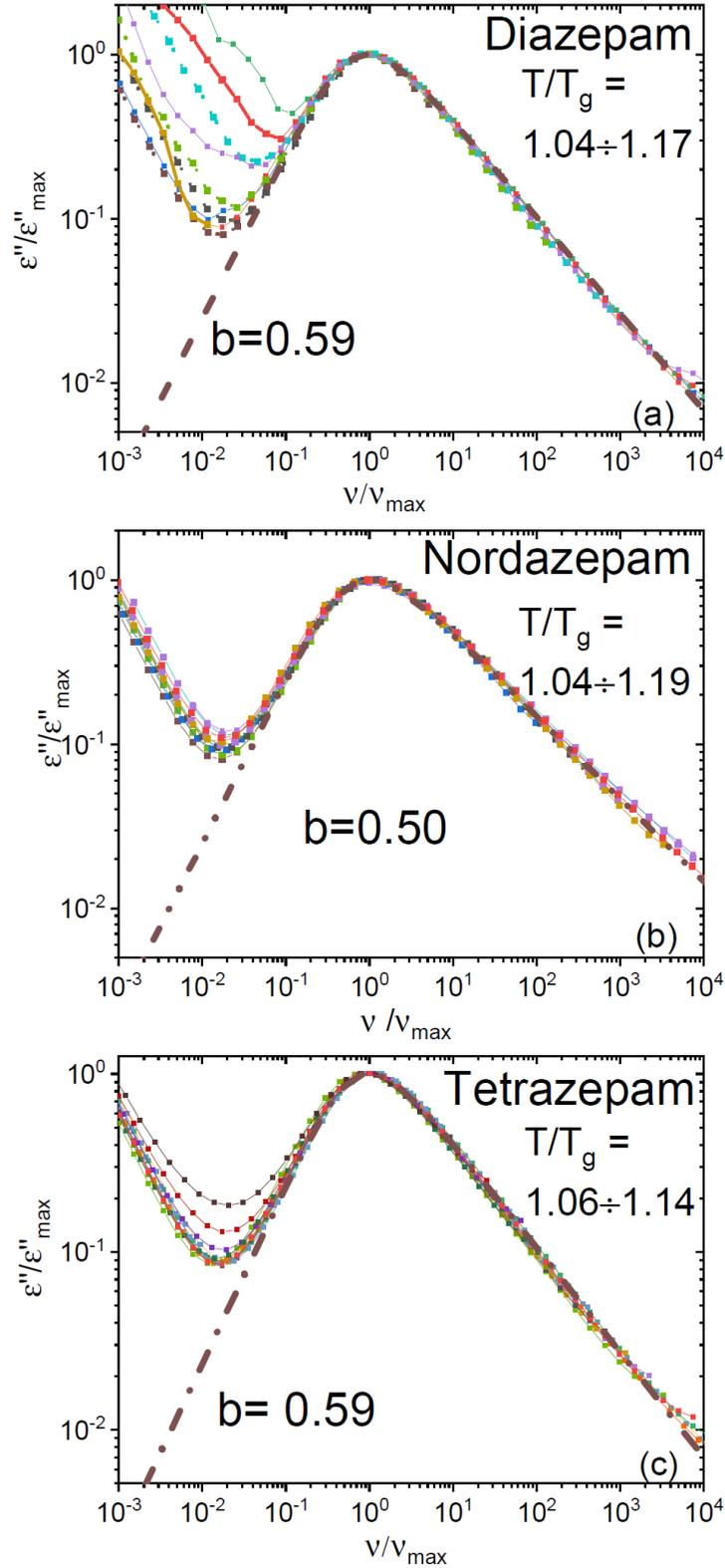
**Figure 5.** BDS spectra of supercooled liquid DIA (a), NOR (b), and TETRA (c), rescaled to the maximum of the  $\alpha$  peak (both in intensity and in frequency). The dashed lines are Cole-Davidson (CD) fits of the  $\alpha$  relaxation component with the indicated CD exponent  $b$ .
