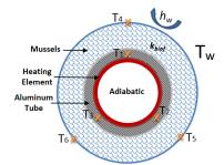
Figure 4: Middle cross-section of the aluminum tube covered with uniform colonization.
