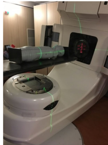
FIG. 2. Radiochromic film placed between slices inside the ATOM dummy (left) and dummy positioning for the 3DCRT treatment (right).
