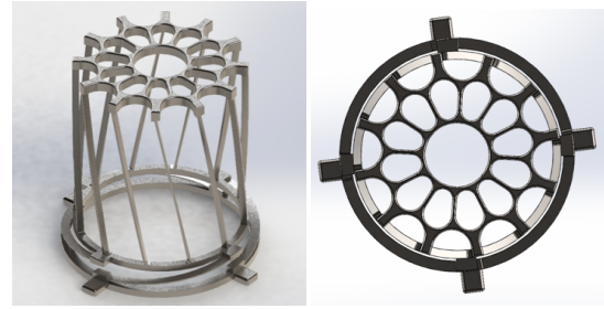
Figure 10: CAD rendering of the adapted, 3D-printable CWM in perspective (left) and top view of the light-weight end plate (right).
