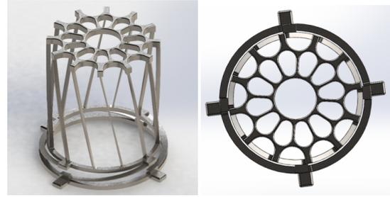
Figure 10: CAD rendering of the adapted, 3D-printable CWM in perspective (left) and top view of the light-weight end plate (right).
