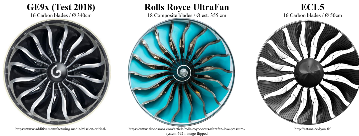
Fig. 2 Low-speed Fan technology demonstrators and Open Test Case ECL5/CATANA
