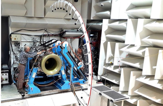
Fig. 3 Fan-Test-Facility with anechoic chamber PHARE-2 (ECL-B3), (Aero/Acoustic/Aeroelastic)
