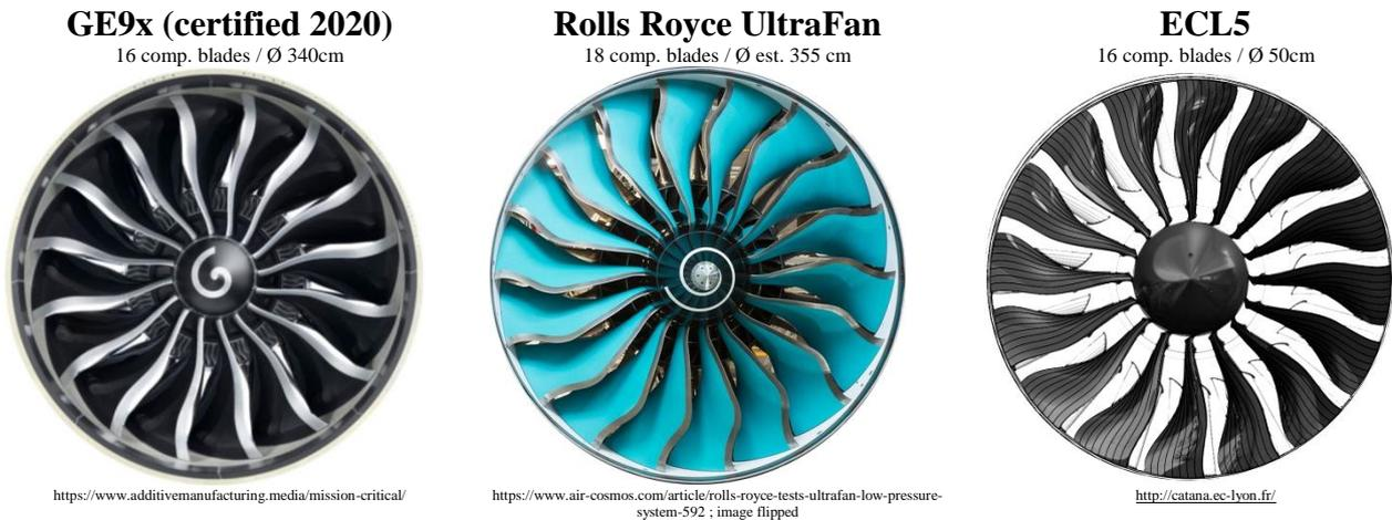
Fig. 2 Modern industrial low-speed composite fans and Open Test Case ECL5/CATANA
