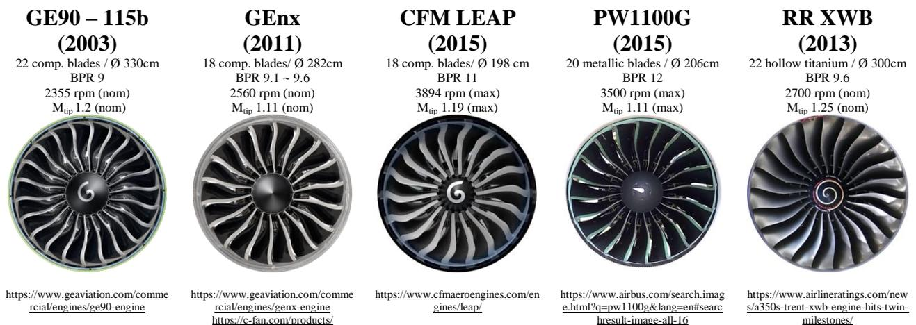
Fig. 1: Selection of established modern High-Bypass-Ratio Engines
