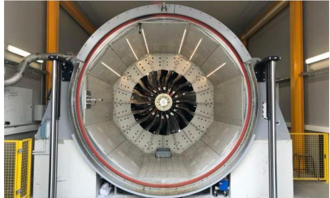
Fig. 4 Vacuum Test Facility PHARE-1 (structural damping)
