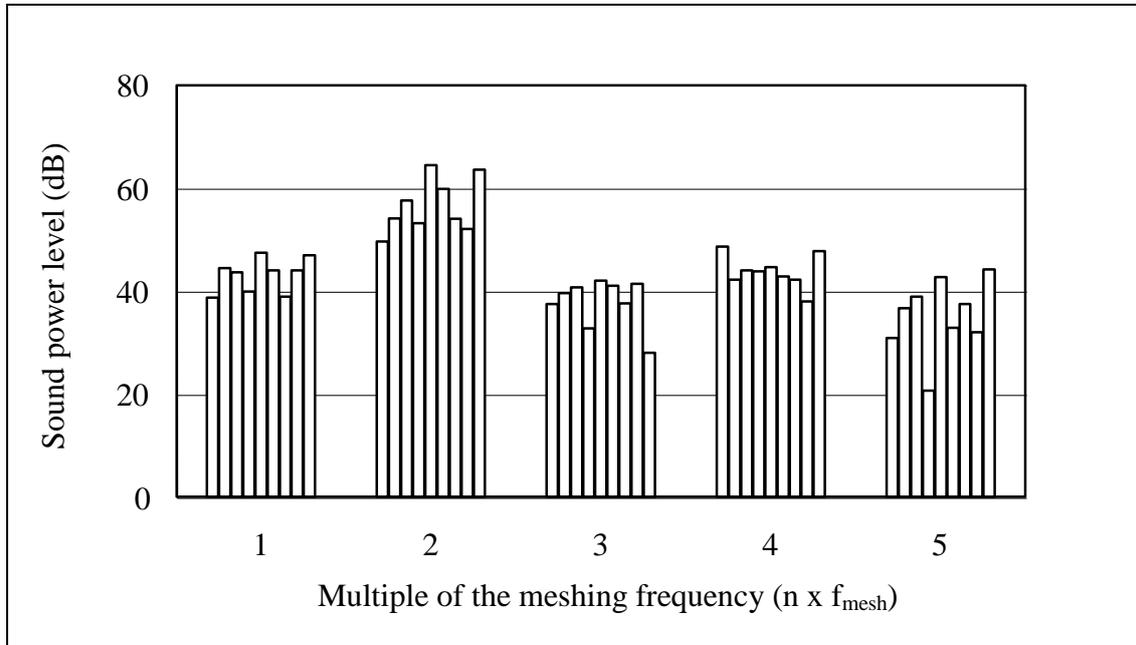
*Figure 6. Spectra of the sound power level for the 9 numerical attempts in increasing order. P8-H8 Configuration.*
