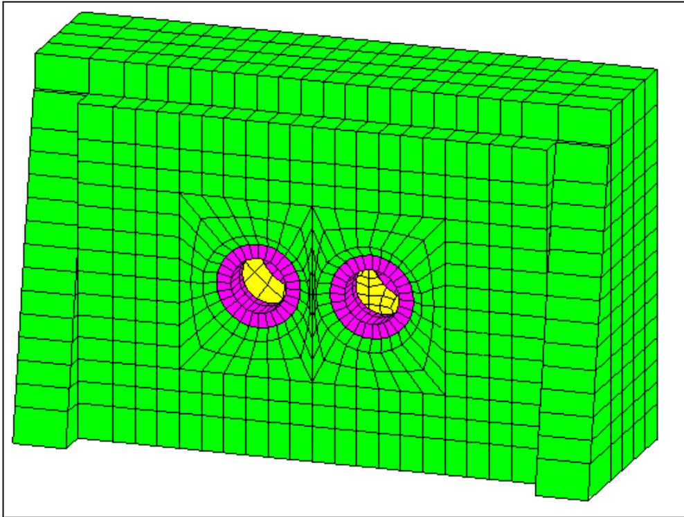
*Figure 2. Finite element modelling of the housing of the studied gearbox. View of the Opposite side.*
