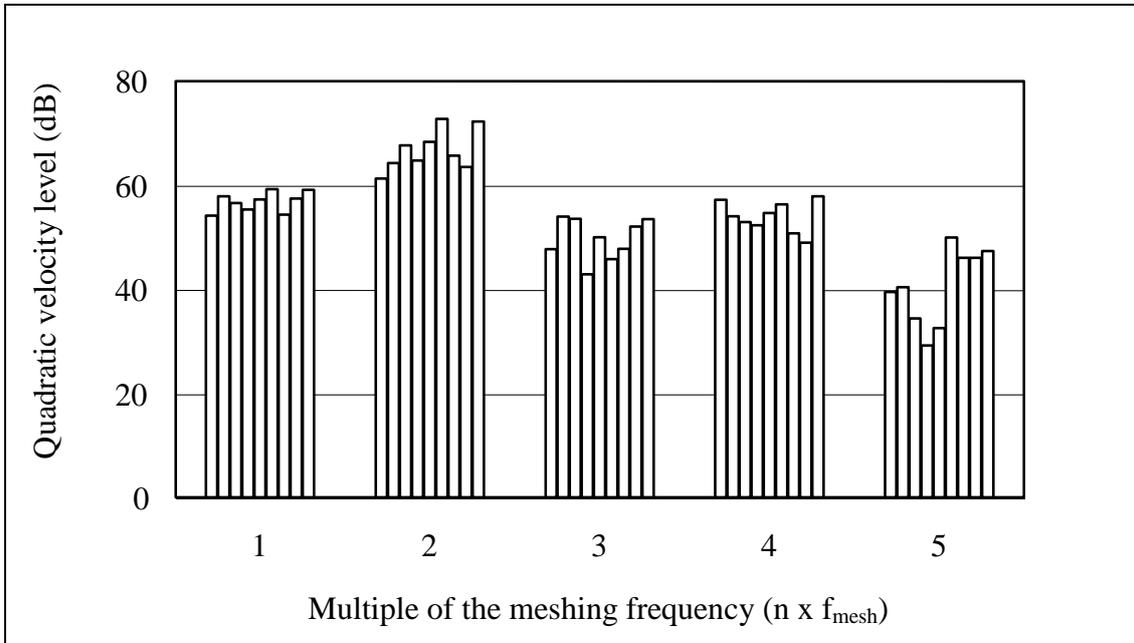
Figure 10. Spectra of the housing quadratic velocity level for the 9 numerical attempts in increasing order. P8-H7 Configuration.
