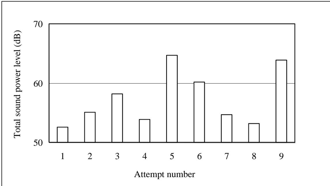
Figure 8. Total sound power level for each of 9 attempts. P8-H8 Configuration.
