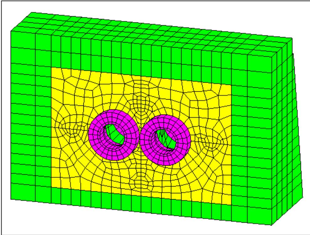
*Figure 1. Finite element modelling of the housing of the studied gearbox. View of the free side.*
