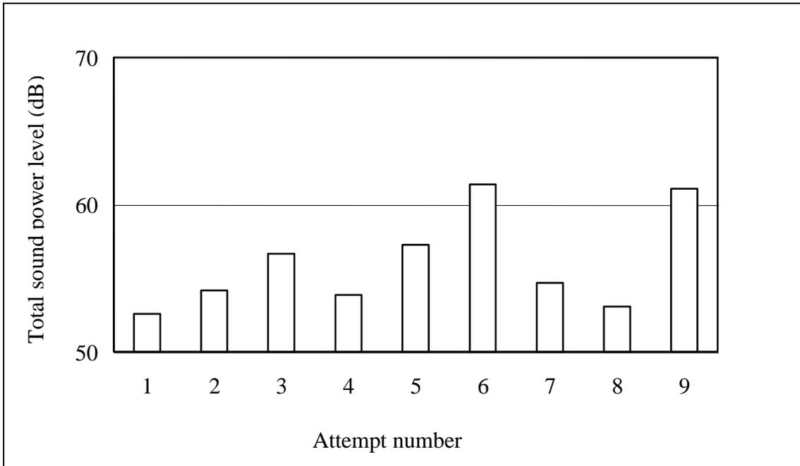
*Figure 12. Total sound power level radiated by the housing for each of the 9 numerical attempts. P8-H7 Configuration.*
