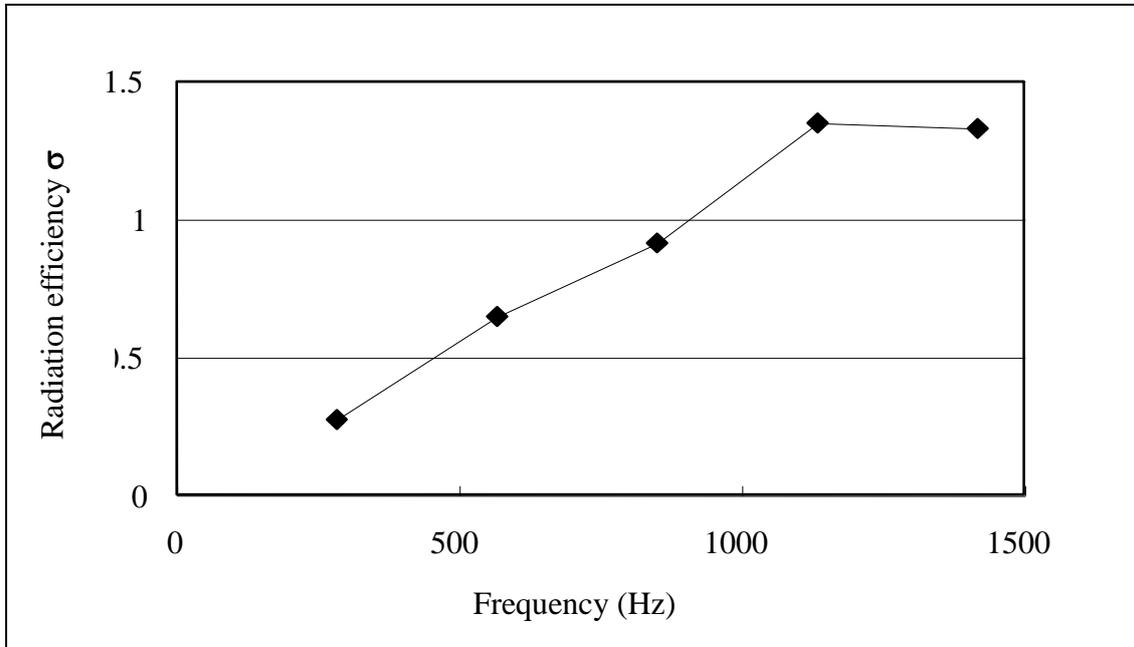
Figure 7. Frequency evolution of the housing radiation efficiency.
