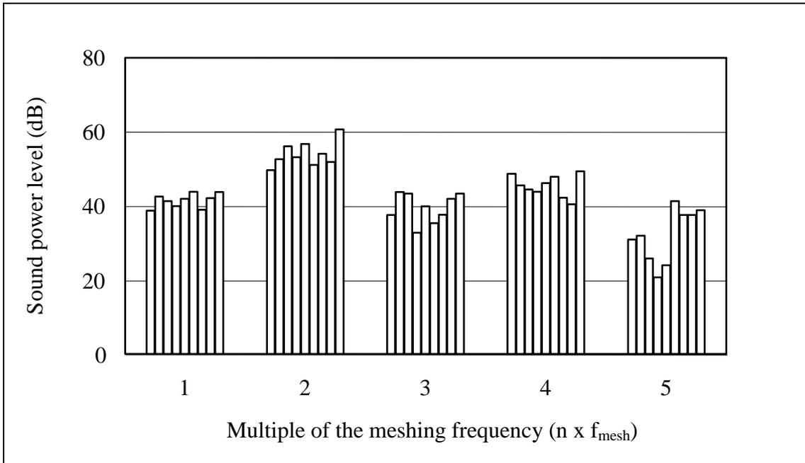
Figure 11. Spectra of the sound power level for the 9 numerical attempts in increasing order. P8-H7 Configuration.
