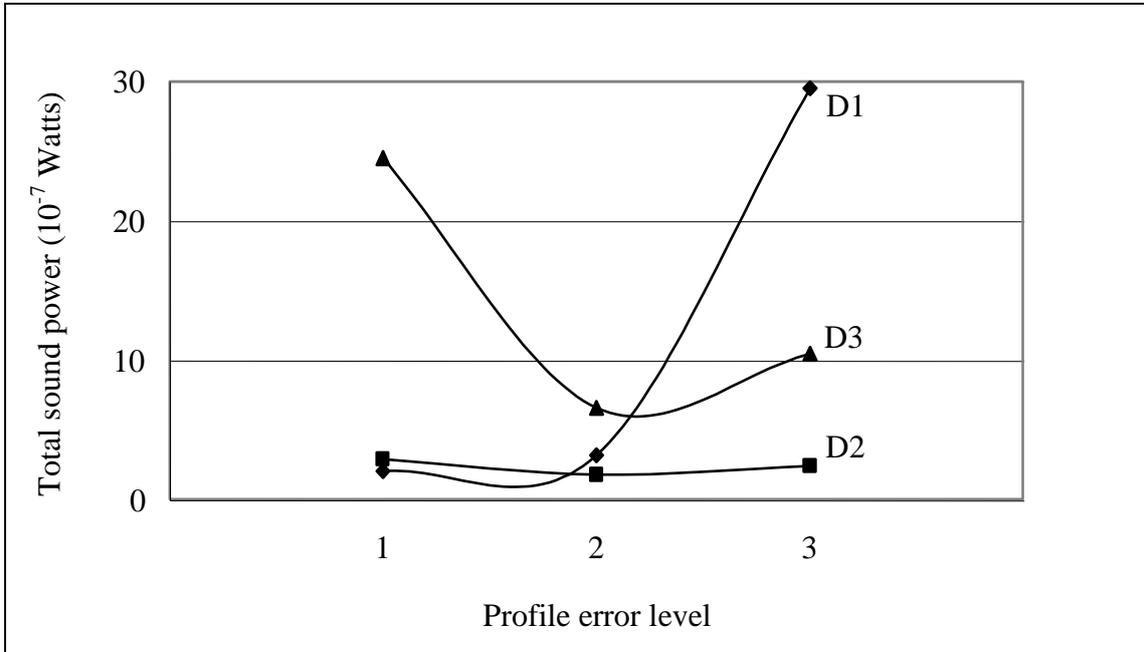
Figure 9. Interaction representation between profile error and helix angle error. P8-H8 Configuration.
