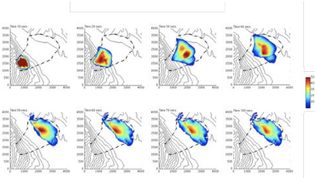
Figure 16: Evolution of the slide using a Pouliquen friction law where  $\delta_1 = 12^\circ$ ,  $\delta_2 = 26^\circ$  and  $d = 1.5\text{m}$ .
