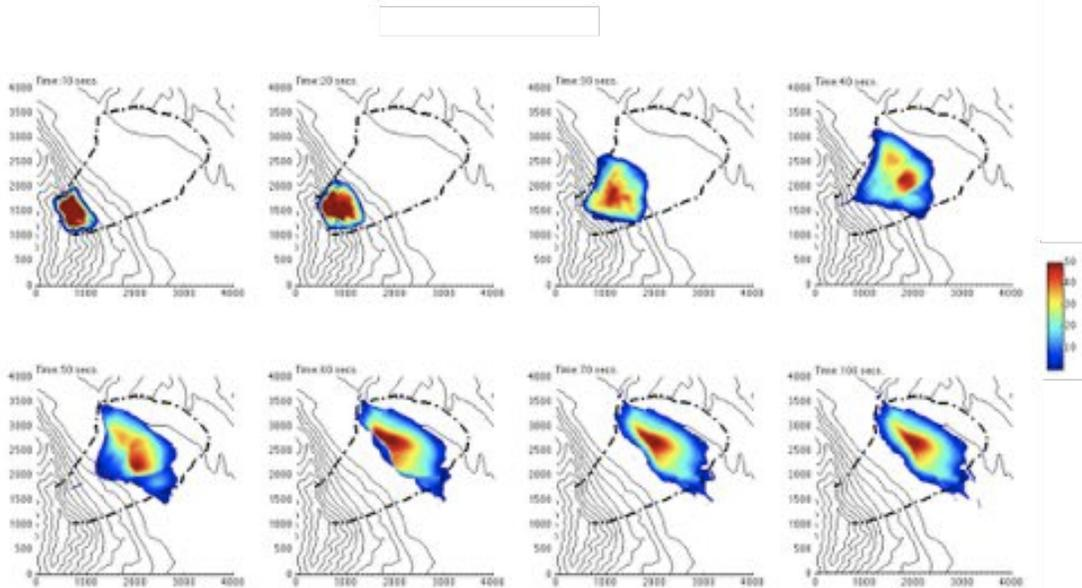
Figure 14: Evolution of the slide using friction angle  $\delta = 14^\circ$ .
