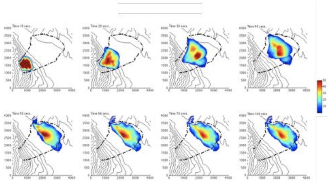
Figure 15: Evolution of the slide using friction angle  $\delta = 12^\circ$ .
