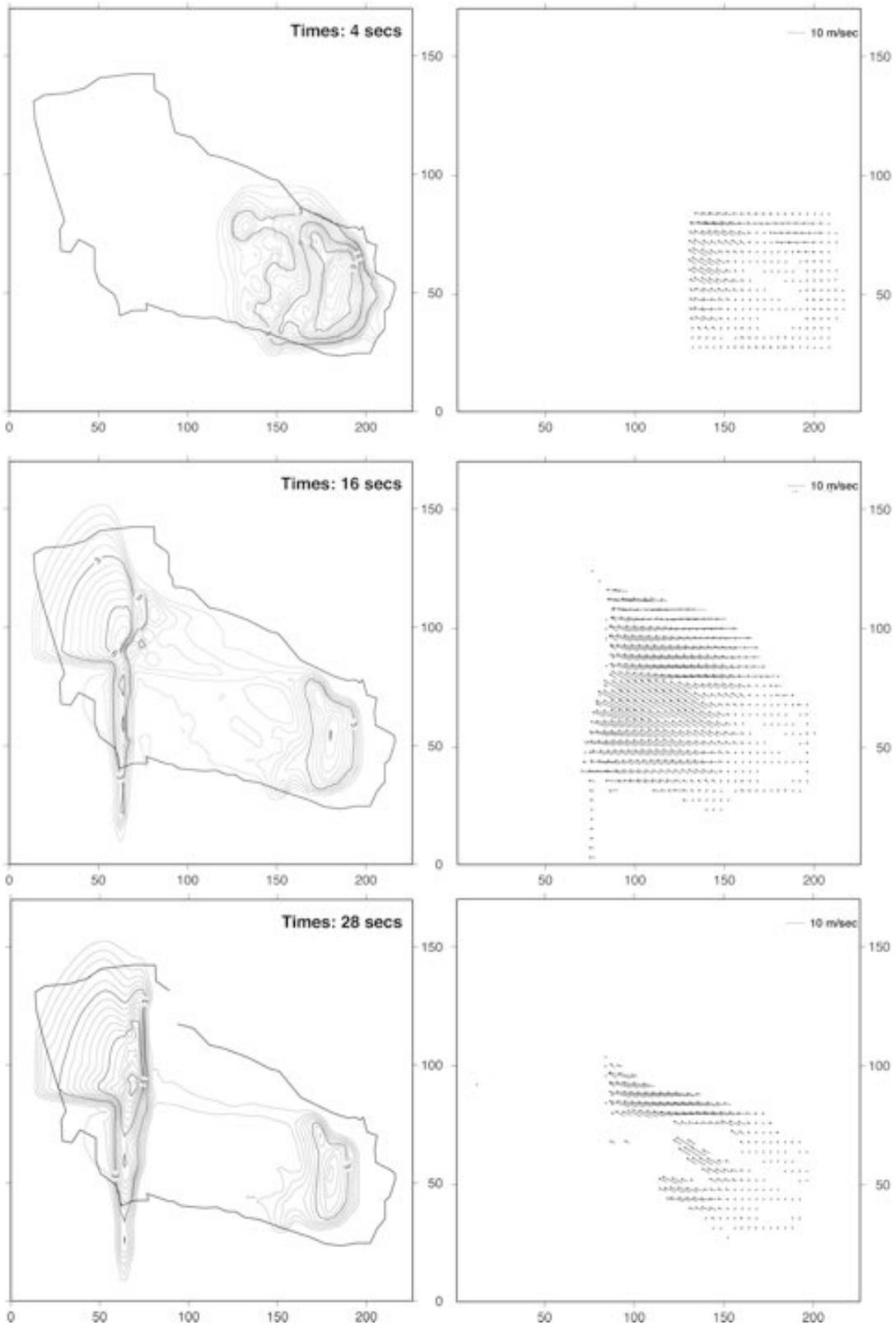
Figure 10: (Left) – Evolution of the mass (Right) – Velocity field. Results from simulation using friction angle  $\delta = 18^\circ$ .
