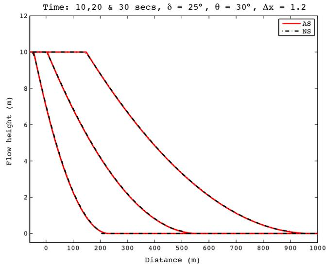
Figure 3: Evolution of the flow height for both analytical and numerical solutions respectively named AS and NS. Using a reasonable space increment  $\Delta x$ , *Shaltop - 2d* is able to reproduce very well the analytical solution.
