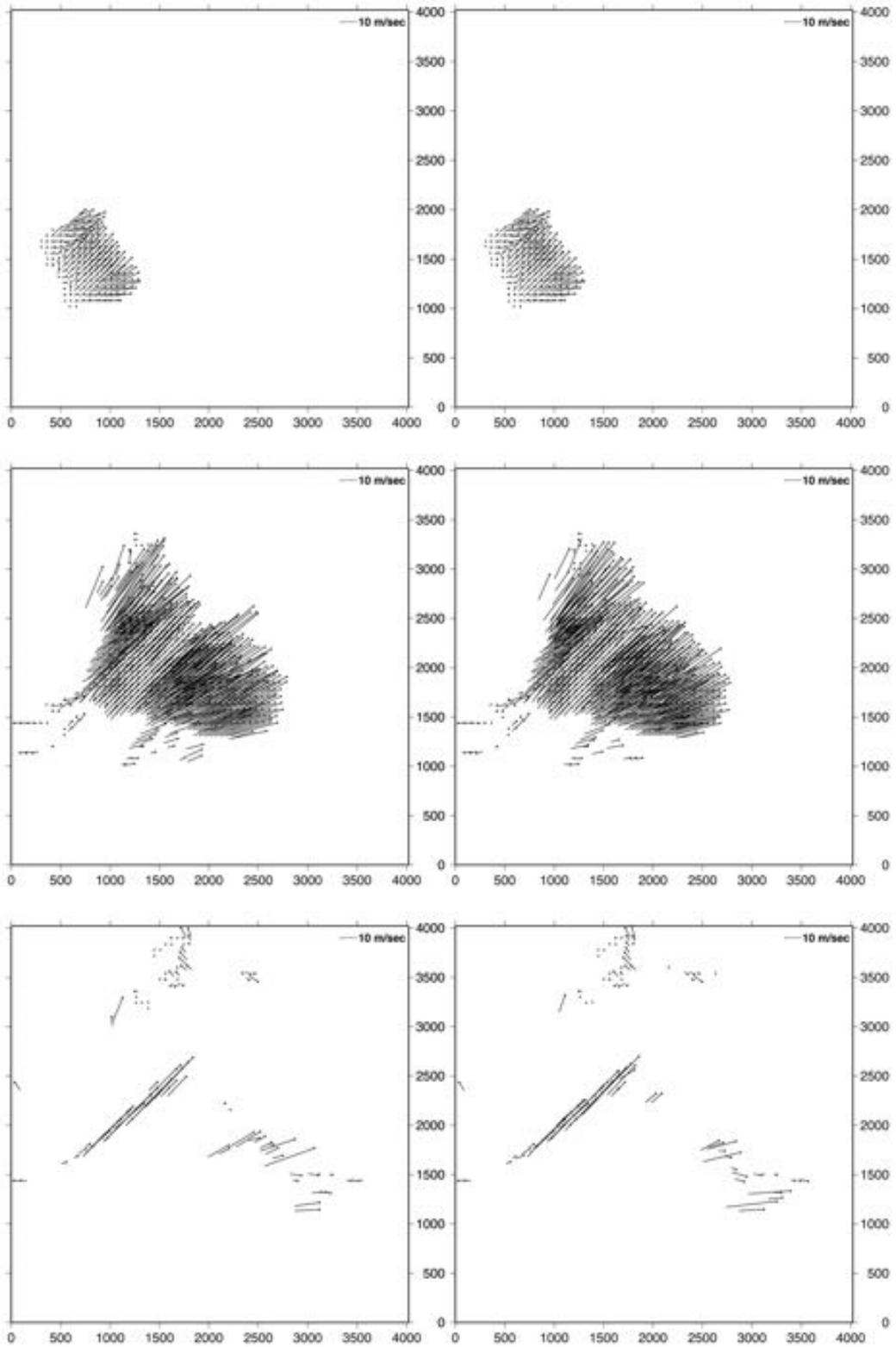
Figure 17: Velocity field at time = 10, 40 and 70 secs. (Left) – Using Coulomb-type friction (Right) – Using Pouliquen-type friction law.
