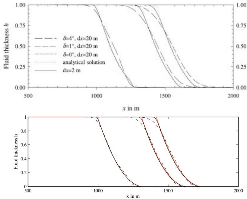
Figure 4: (Top) – Comparison between *RASH<sup>3D</sup>* model with analytical solution (figure from *Mangeney et al.*, 2003). (Bottom) – Using the same parameters, we compare here *Shaltop - 2d* with analytical solution.
