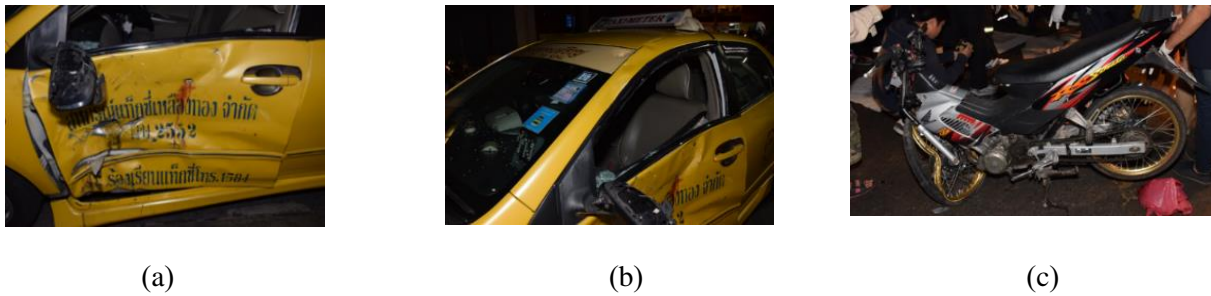
Figure 3. Illustrates (a) deformed door (b) windshield crack (c) deformed front wheel and handle bar
