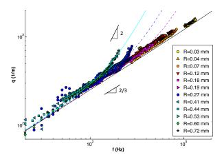
FIG. 3: Dispersion relation of the transverse wave on the PB for different radius R. The lines correspond to Eq. (15) without any fitting parameter. Black solid line: R=0.03 mm, magenta dotted line: R=0.18 mm, blue dashed line: R=0.27 mm and cyan solid line: R=0.41 mm. The typical power laws  $q\sim f^{2/3}$  and  $q\sim f^2$  are indicated on the graph.
