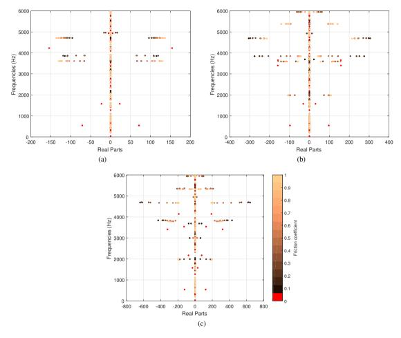
Fig. 4: Evolution of complex eigenvalues in the complex plan assuming a variation of the friction coefficient at the interfaces for three different values of  $\mu_{pad-disc}$ : (a)  $\mu_{pad-disc} = 0.3$ , (b)  $\mu_{pad-disc} = 0.5$  (c)  $\mu_{pad-disc} = 0.7$
