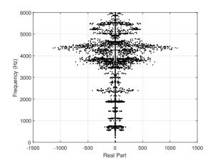
Fig. 5: Complex eigenvalues for all configurations considered
