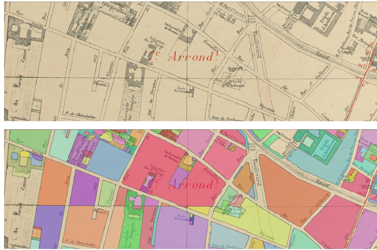
Fig. 1: Example (cropped) of a raster map used as input (top) and output of our vectorization approach (bottom): a set of individual polygons in vector format ready for further annotation in any GIS software. Some shapes are still undetected.
