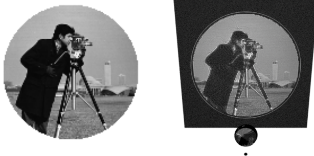
Figure 2: Left: target image. Right: simulation of the scene using the appleseed ® rendering engine; the small black disk at the bottom represents the light source.
