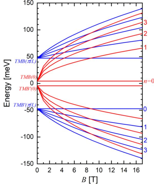
**Figure 6. Landau levels of the topological minibands.** Calculated Landau levels of  $TMB$  and  $TMB'$  at  $q_z = 0$  (red) and  $q_z = \pm \pi/L$  (blue). Calculations have been performed with the parameters  $d_{QW} = 9$  nm;  $d_B = 3.5$  nm;  $2\Delta_{QW} = -72.5$  meV;  $2\Delta_B = +150$  meV and  $v_{\parallel} = v_z = 4.40 \times 10^5$  m/s. Some Landau level indexes  $n$  are written at the right.
