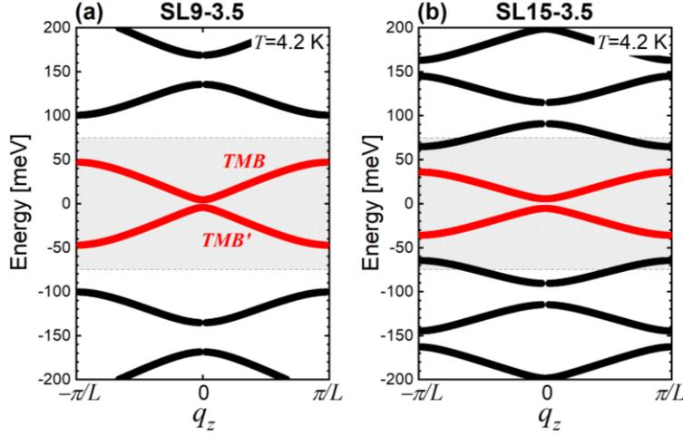
**Figure S1.** Miniband dispersions of SL9-3.5 and SL15-3.5 at  $T=4.2$  K. In red are the calculated  $TMB$  and  $TMB'$  and in black are the higher excited minibands. The grey area indicates the barrier potential height.
