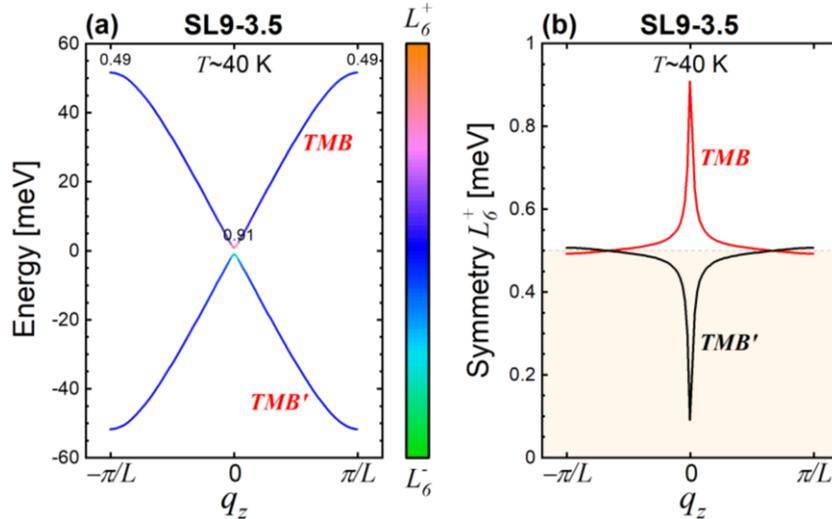
**Figure S2.** (a) Miniband dispersion for SL9-3.5 similar as Fig. 2(b) of the main text, but for  $T \sim 40$  K, where the SL gap is negative but nearly zero, illustrating the case where the band inversion does not occur over the whole mini BZ but only in a very narrow region around  $q_z = 0$  (see color scale and labels which denote the  $L_6^+$ -parity). (b) Calculated  $L_6^+$ -parity of  $TMB$  and  $TMB'$  shown in (a). The miniband is only partially inverted around  $q_z = 0$ .
