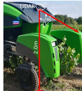
Fig. 3: LiDAR-sensor's position on top of the robot.
