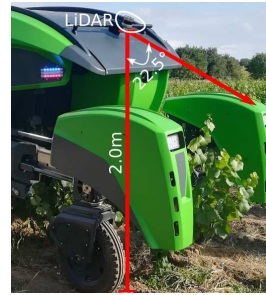
Fig. 3: LiDAR-sensor's position on top of the robot.
