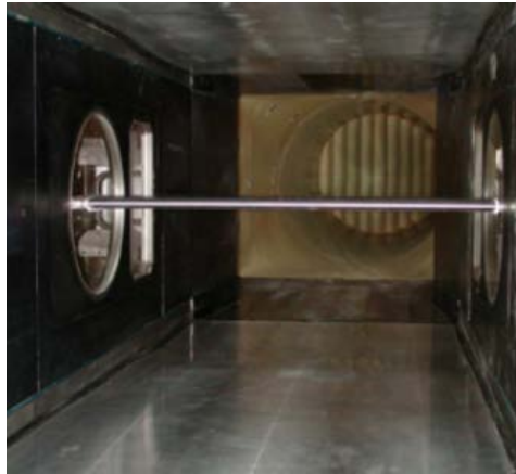
Figure 10: Picture showing the OALT25 airfoil installed in the test section of the S3Ch wind tunnel. View from upstream.
