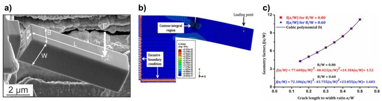
Fig. 10: (a) SEM image of a fractured cantilever in a NiAl single crystal, (b) FE model for the determination of the geometry function, shown in (c) for different  $a/W$  aspect ratios [57].
