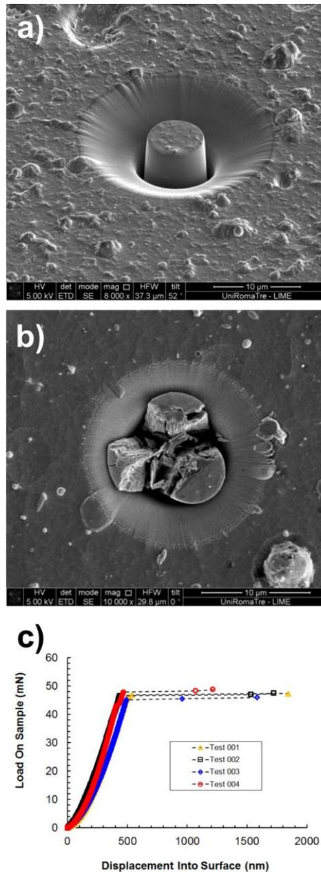
Fig. 2: (a) Example of a CrAlN/Si<sub>3</sub>N<sub>4</sub> pillar before splitting. (b) Example of a CrN pillar after splitting. (c) Load-displacement curves for CrN pillars, highlighting the critical load ( $P_c$ ) corresponding to the crack 'popping out' to the side surface, and pillar splitting [31].
