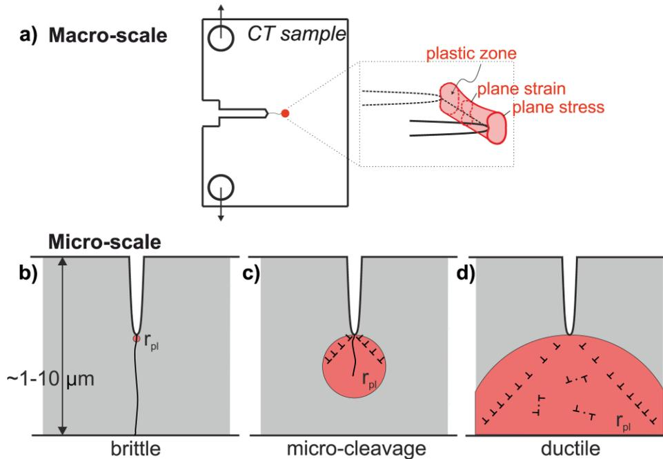
*Fig. 15: Schematics for the description of the plastic zone ahead of the crack tip (a) in a compact tension specimen and in a single crystal (SX) micron-scale specimen showing (b) brittle fracture, (c) dislocation-controlled micro-cleavage and (d) an entirely ductile behaviour with dislocation nucleation from the crack tip and from active sources.*
