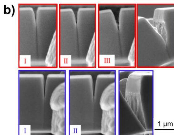
Fig. 21: (a) Force-CMOD curves for the hard and soft orientation and (b) corresponding SEM images. The soft orientation showed brittle fracture whereas a constant force plateau was obtained for the hard orientation. The begin of the force plateau (II) was taken as final data point for the determination of  $v_{pl,hard}$ . Note the apparent crack growth from image (II) to (III). After testing, the samples were tilted to allow for an inclined observation of the fracture surfaces.
