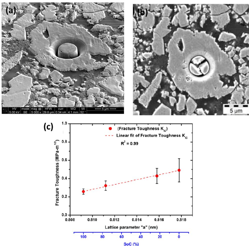
Fig. 8: (a,b) FIB-milled micro-pillars before and after splitting of Li<sub>x</sub>Mn<sub>2</sub>O<sub>4</sub> crystals embedded in polymeric matrix; (c) fracture toughness as a function of lattice parameter [39].
