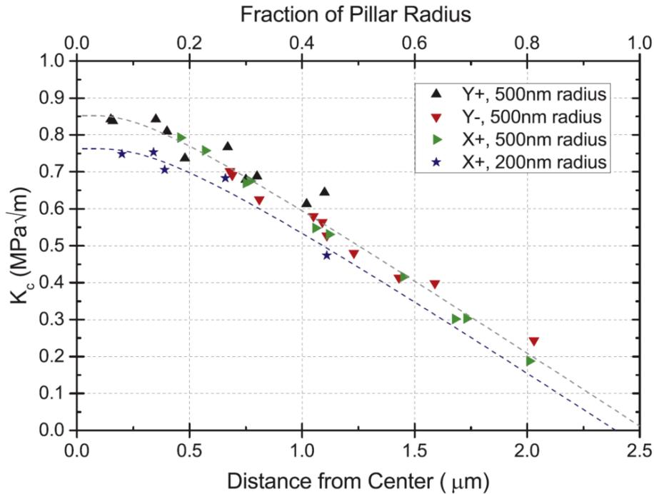
Fig. 5: Apparent fracture toughness as a function of distance to the center of the pillar with the offset orientation direction and the indenter tip radius noted [36].
