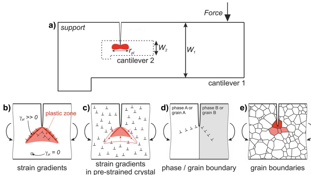
*Fig. 16: The development of plastic zones in loaded micro-cantilevers: (a) although cantilever size may change, plastic zone size remains the same for given severity of loading, (b) strain gradient effects, (c) effect of additional plastic pre-straining, (d) testing of single phase or grain boundaries and (e) testing of multiple grains; after [65].*
