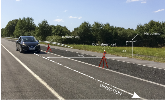
Figure 5: Experimental set-up for CPB noise tests, here exemplified in the case of the Nissan LEAF rolling on test section E1
