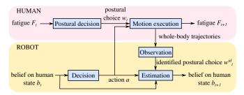
Fig. 1: Workflow of the human-robot interaction process during the execution phase, according to the proposed model. The robot decision follows the precomputed policy  $\pi$ .
