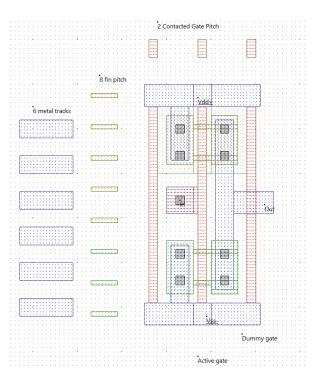
Figure 36: design of a high density 2-fin inverter using a 6-Track design (inv 2Fin.MSK)
