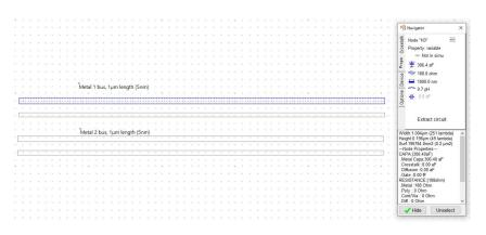
Figure 31: Extracting the R & C values from a metal 1 bus, minimum width & spacing, length 1µm (metal-1um.MSK).
