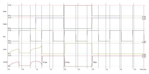
Figure 48: Write & Read cycles at VDD=0.25V
