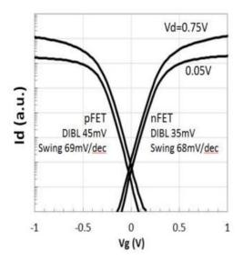
Figure 18: 5-nm Id/Vg characteristics presented in arbitray units [Yeap 2019]
