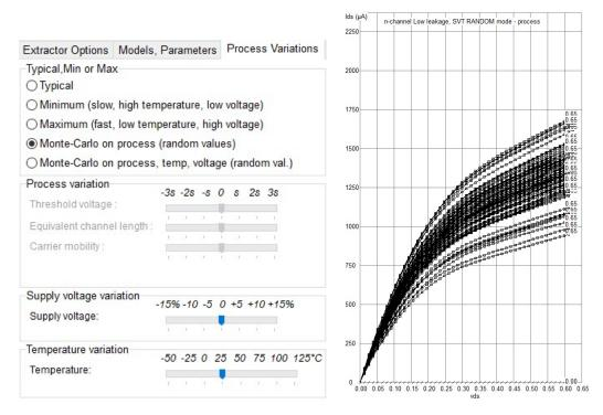
*Figure 27: Plot of 100 Id/Vd with normal distribution of threshold voltage, effective width and channel mobility showing a spread in performances*
