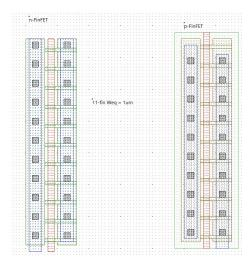
Figure 19: designing a FinFET with 1µm-eq. width would require 11 fins (finFET-5nm-Weq1um.MSK)
