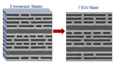
*Figure 12 : One Extreme UltraViolet (EUV) may replaces 5 immersion masks, with better patterning yield & shorter fabrication time [Yeap 2019]*
