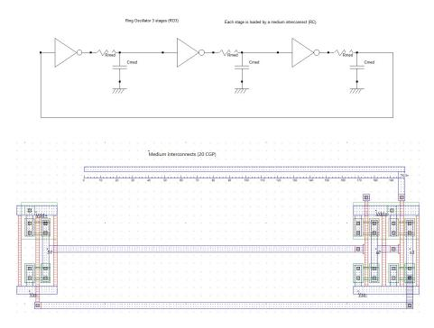
Figure 41: medium interconnects around 20 CGP (800 nm, RO3-FO1-Medium.MSK)
