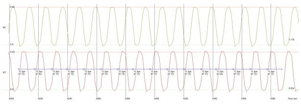
Figure 39: Simulation of the Ring Oscillator with FO3 (RO3-FO3.MSK) reaching 90 GHz
