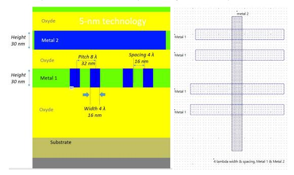
Figure 29: metal1, metal2 interconnect cross section & upper view, metal pitch 8  $\lambda$  (32 nm)
