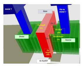
Figure 16: Illustration of Fin thickness, length & pitch
