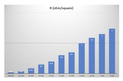
Figure 30: The resistance per square (log scale) of lower metal layers vs. technology
