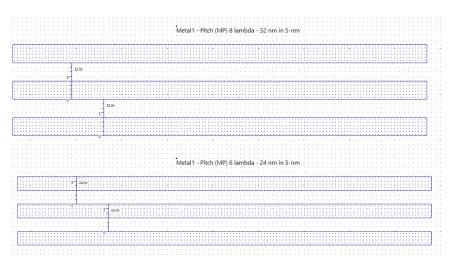
*Figure 10: Illustration of metal width, spacing & pitch for two variants: minimum pitch 24 nm & regular pitch 32nm used for automatic routing (5nm\metal pitch.MSK)*
