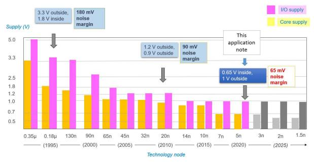
Figure 11 : Illustration of the supply voltage reduction with feature size reduction over 30 years of technology progresses
