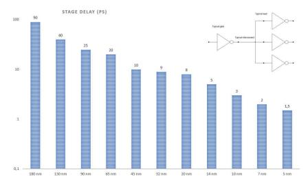
Figure 5: Average switching delay per gate for technologies ranging from 0.18  $\mu$ m down to 5 nm
