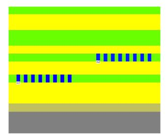
*Figure 13: Cross-section of a metal bus in metal 1 (left) and metal 2 (right) with a 32-nm lower metal pitch*
