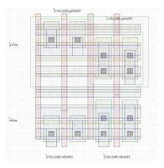
Figure 34: Adding FinFETs to the routing grid (routing grid finFets.MSK)
