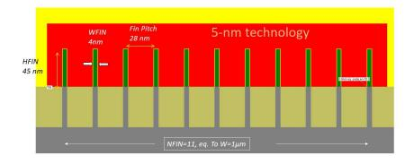
Figure 20: Cross-section of the FinFET with 1µm-eq. width with 11 fins (finFET-5nm-Weq1um.MSK)
