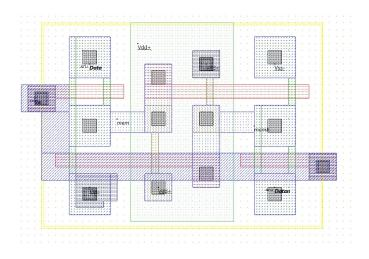
Figure 46: design of a 6T 2-fin static RAM (sram-6T-HD-5nm.msk)
