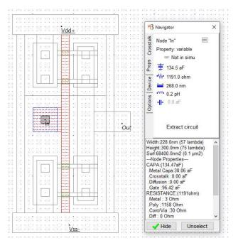
Figure 21: extracting the input capacitance of an inverter (inv.MSK)
