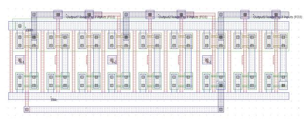
Figure 38: Design of Ring Oscillator, each stage with 3 inverter gates connected to its output, gate 2 fins, gate pitch 44 nm (RO3-FO3.MSK)
