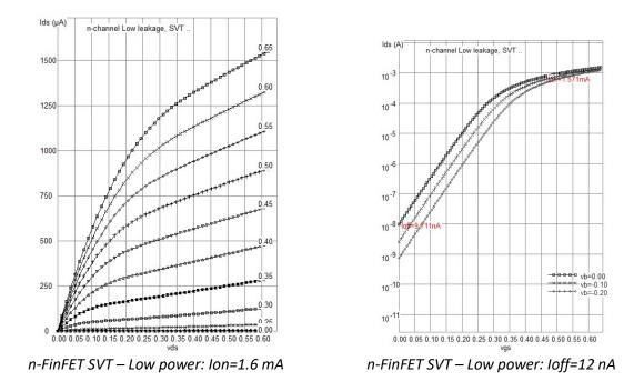
Figure 24: n-FinFET Low Power, standard VT=0.3V, Ion=1.6mA, Ioff=10nA @ VDD=0.65 V
