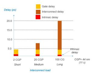
Figure 42: delay increase with interconnect length (metal1, 4  $\lambda$  width)
