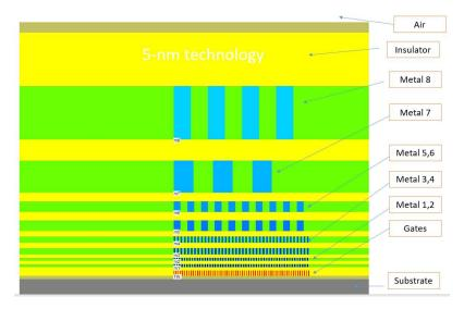
Figure 28: cross-section showing 8 metal layers (All metals 5nm.MSK)
