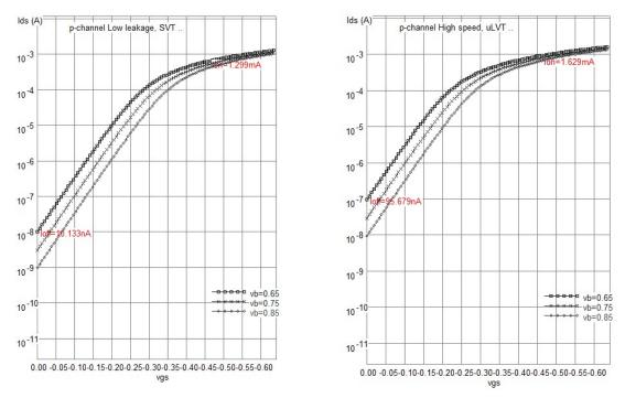
Figure 26: p-FinFET SVT : Ion=1.6mA, Ioff=14nA; p-FinFET uLVT: Ion=1.6mA, Ioff=100nA @ 0.65 V
