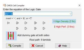
Figure 43: The cell compiler is us ed to generate cells automatically
