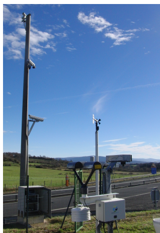
Figure 2. The recording station at the Col de la Fageole (A75 highway, France). The site is instrumented with a camera and weather sensors.
