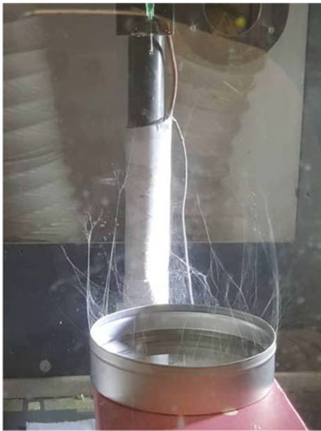
Fig. 4 Image showing standing fibers on the collector from electrospinning of 4 % CP in DBU-CO 2 switchable solvent system (E-spinning conditions: 29Kv-20 cm-0.12ml/hr)
