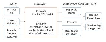
Fig. 1. Schematic view of the Tradcare flow
