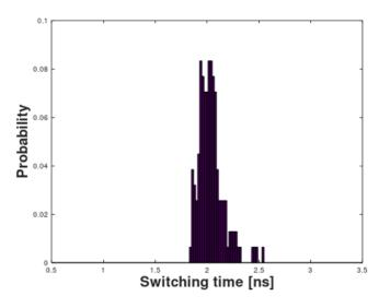
Fig. 4. Switching probability distribution at 1 V for 10 nm radius STT- MTJ
