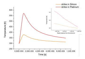
Fig. 7. Xe on Si and Pt: Thermal spikes at 30 nm from the hit point, Inset: maximum propagation range in Si and Pl.
