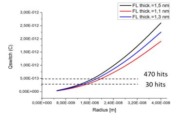
Fig. 3. Free layer Critical charge by varying MTJ radius and FL thickness
