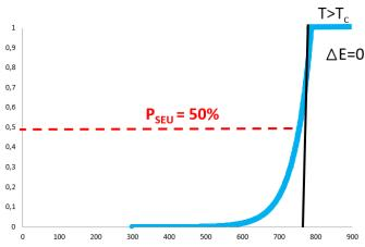
Fig. 8. Free layer thermal switching probability distribution after a time t= 5 ns at different temperatures
