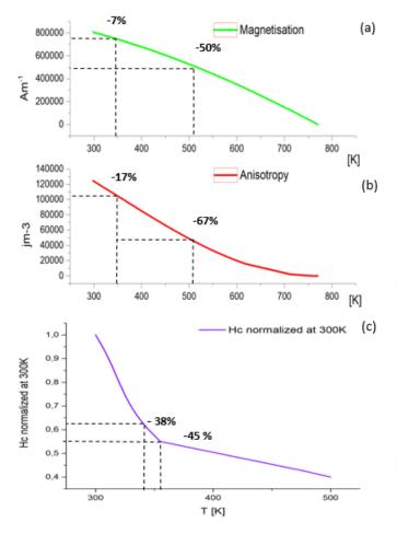
Fig. 9. Temperature variation of Magnetization (a), Anisotropy (b) and Coercive field (c)
