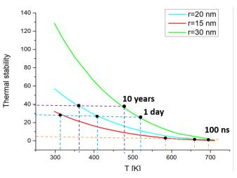
Fig. 10. Thermal stability factor and retention time impacted from scaling and temperature rise
