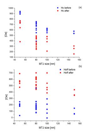
Fig. 11. Variation of coercive field and offset field post 200°C annealing
