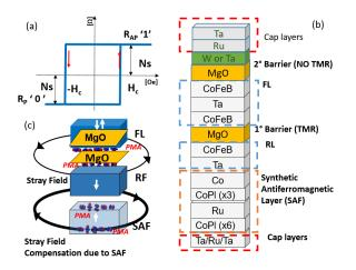
Fig. 2. Hysteresis loop of the Free Layer:  $H_c$  represent the coercive field,  $N_s$  the number of spin polarized electrons (a). Typical double-interface CoFeB/MgO stack of a STT-MTJ (b). Simplified view of the three main blocks which constitute the STT-MTJ.
