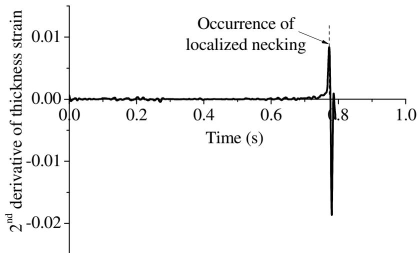
**Fig. 9.** Prediction of localized necking based on the maximum of the 2<sup>nd</sup> derivative of thickness strain.
