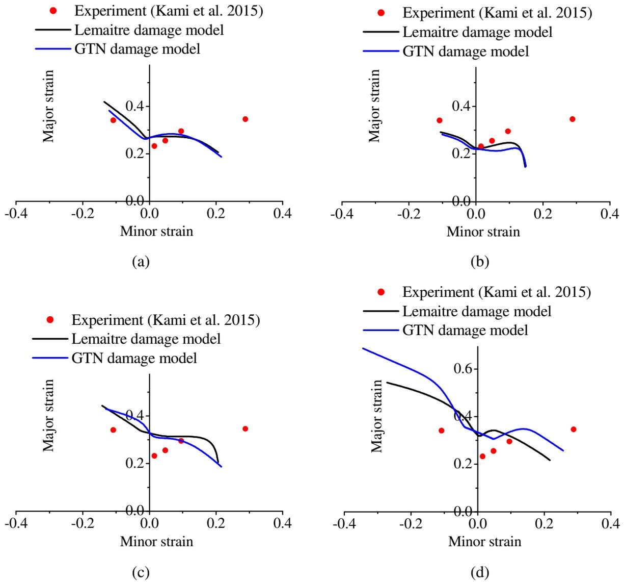
**Fig. 13.** Prediction of FLDs using the four localized necking criteria: (a) maximum of the 2<sup>nd</sup> derivative of thickness strain, (b) ratio of equivalent plastic strain increment, (c) maximum of punch force, and (d) loss of ellipticity.
