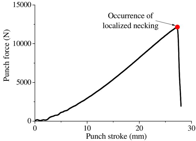
**Fig. 11.** Prediction of localized necking based on the maximum in the punch force–displacement response.
