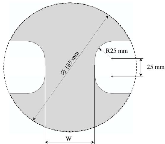
**Fig. 3.** Specimen geometry and dimensions used in the Nakazima deep drawing test.
