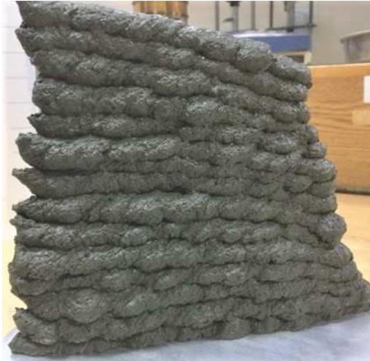
Figure 1: Manually printed element using Mix A for printability assessment
