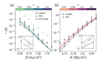
FIG. 2. Mean waiting time between reversals at 300 K,  $\tau$ , as a function of the (a) DMI, D, and (b) anisotropy, K, computed with Langer's theory and FFS for different values of the Gilbert damping,  $\alpha$ . The insets give a comparison between Langer's theory and the estimate based on  $f_0 = 1$  GHz. In (a), a single run with full dipole-dipole interactions (DDI) is also shown.
