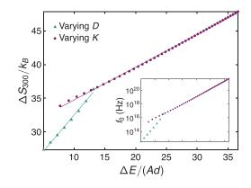
FIG. 4. Activation entropy at T=300 K,  $\Delta S_{300}/k_B$ , computed with Eq. (6), as a function of the activation energy normalized by the characteristic exchange energy,  $\Delta E/(Ad)$ , for variations in D and K. Solid lines represent linear fits to the data. The inset shows the corresponding variation of  $f_0$  for  $\alpha = 0.5$  with the same horizontal scale.
