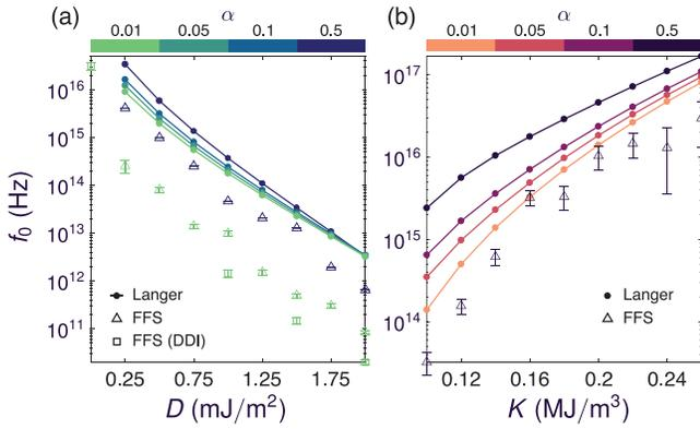
FIG. 3. Arrhenius prefactor,  $f_0$ , as a function of the (a) DMI,  $D$ , and (b) anisotropy,  $K$ , computed with Langer's theory and FFS for different values of the Gilbert damping,  $\alpha$ . Points involving full dipole-dipole interactions (DDI) were obtained with energy barriers from Ref. 23.
