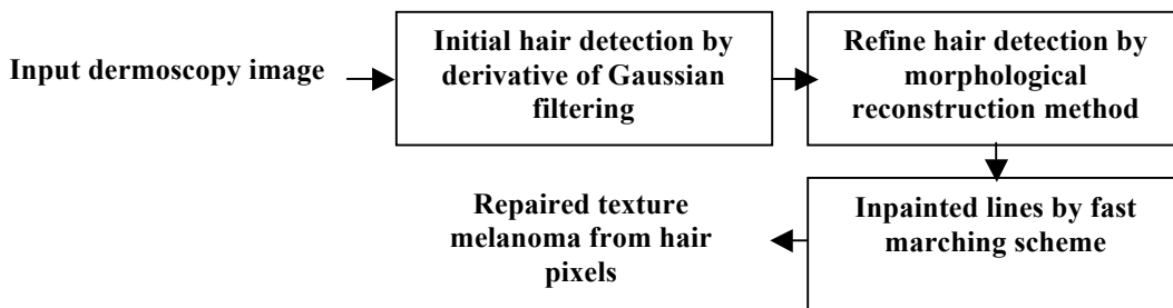
Figure 1. Systematic flow diagram of the proposed hair-occluded information repair algorithm.
