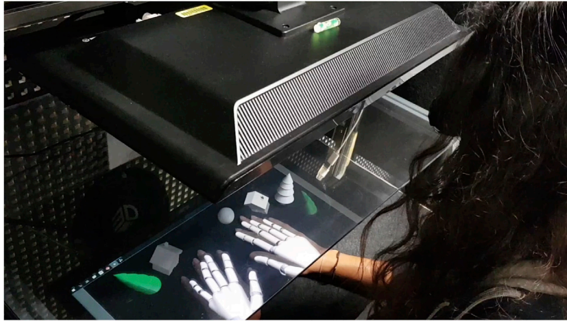
FIGURE 1 | The experimental setup. A user equipped with tracked shutter glasses looks at her virtual hands under the semi-transparent mirror. The rendered perspective of the holograms is adapted to her point of view in real-time. For illustration clarity, we colored two of the virtual trees in a distinct color (green) from the real objects (white). All objects were white during the experiment.
