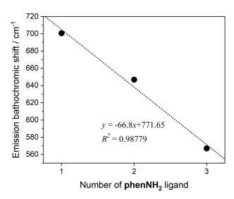
**Figure 9.** Bathochromic shift observed for the emission of  $[Ru(Phen)_{3-n}(Phen-NH_2)_n](PF_6)_2$  (in cm<sup>-1</sup>) from dichloromethane to DMSO, according to the number n of phen-NH<sub>2</sub> ligand(s).
