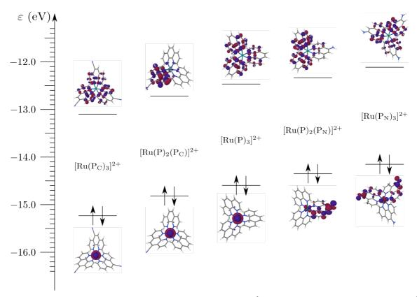
**Figure 3**. Calculated HOMO and LUMO levels of the homoleptic  $[Ru(L)_3]^{2+}$  (L = P, P<sub>C</sub>, P<sub>N</sub>) and heteroleptic  $[Ru(P)_2(L)]^{2+}$  (L = P, P<sub>C</sub>, P<sub>N</sub>) complexes (P = phen, P<sub>C</sub> = phen-CN, P<sub>N</sub> = phen-NH<sub>2</sub>; iso-surfaces calculated for isovalues of  $\pm 0.04$  au; SAOP/TZ2P results).
