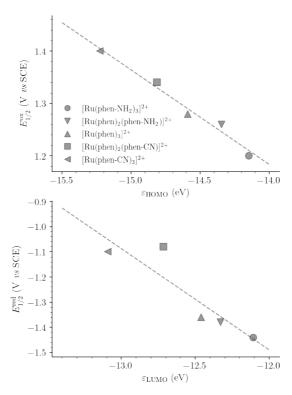
**Figure 4**. Plots of the first oxidation and reduction potentials of [Ru(phen-CN)<sub>3</sub>]<sup>2+</sup>, [Ru(phen)<sub>2</sub>(phen-CN)]<sup>2+</sup>, [Ru(phen)<sub>2</sub>(phen-NH<sub>2</sub>)]<sup>2+</sup> and [Ru(phen-NH<sub>2</sub>)<sub>3</sub>]<sup>2+</sup> as functions of their calculated HOMO and LUMO energies, respectively. The dashed lines correspond to the results of linear least-square regression calculations
