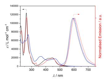
Figure 5. Absorption in molar extinction coefficient and normalised luminescence spectra at room temperature ( $\lambda_{exc}$  = 450 nm), in acetonitrile of homoleptic complexes [Ru(phen)<sub>3</sub>](PF<sub>6</sub>)<sub>2</sub> (black/grey), [Ru(phen-CN)<sub>3</sub>](PF<sub>6</sub>)<sub>2</sub> (blue/light blue), and [Ru(phen-NH<sub>2</sub>)<sub>3</sub>](PF<sub>6</sub>)<sub>2</sub> (red/light red).
