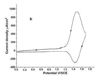
**Figure 2.** a *top*: Repeated cyclic voltammograms from 0.8 to 1.7 V vs. SCE of  $[\mathbf{Ru}(\mathbf{phen-NH_2})_3]^{2+}$  in CH<sub>3</sub>CN/0.1M Bu<sub>4</sub>NPF<sub>6</sub> on platinum electrode; **b** *bottom*: Cyclic voltammogram of the platinum electrode coated with the film poly- $[\mathbf{Ru}(\mathbf{phen-NH_2})_3]^{2+}$  in fresh electrolyte solution.
